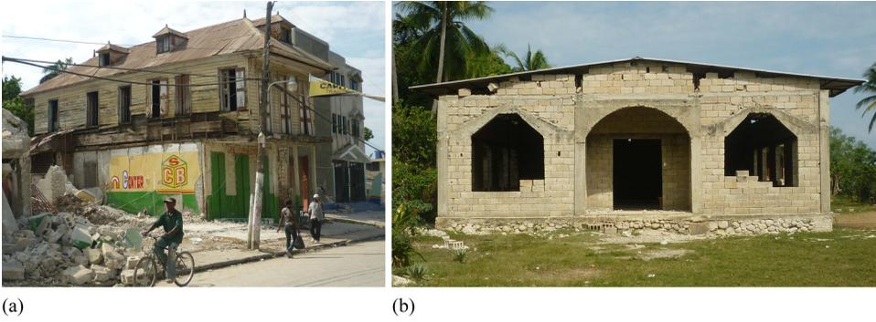
**Figure 8.** Light buildings that were damaged but did not collapse: (a) Wood-frame building, and (b) church with masonry walls and light-metal roof.
