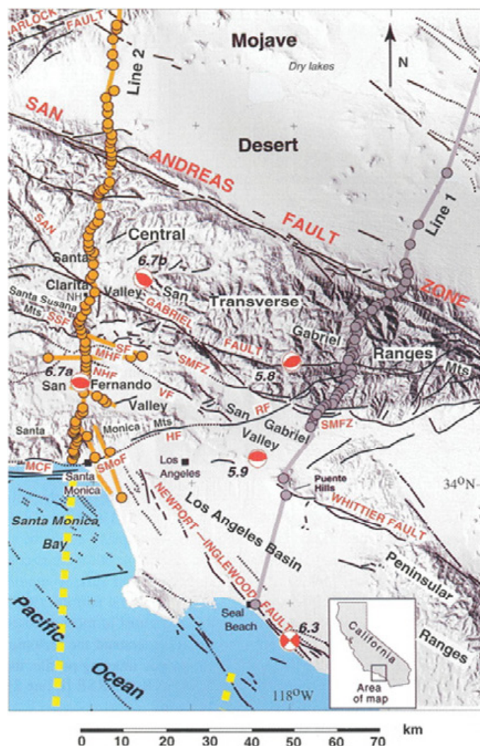
Figure 9.4.2-19. Shaded relief map of the Los Angeles region, southern California, showing location of the LARSE active source seismic profiles (from Fuis et al., 2003, fig. 1). Small circles—shotpoints; colored lines—seismic recording stations; yellow dashed lines—airgun pulses; large red circles—epicenters of large earthquakes (with focal mechanisms and magnitudes). [Geology, v. 31, p. 171–17. Reproduced by permission of the Geological Society of America.]
