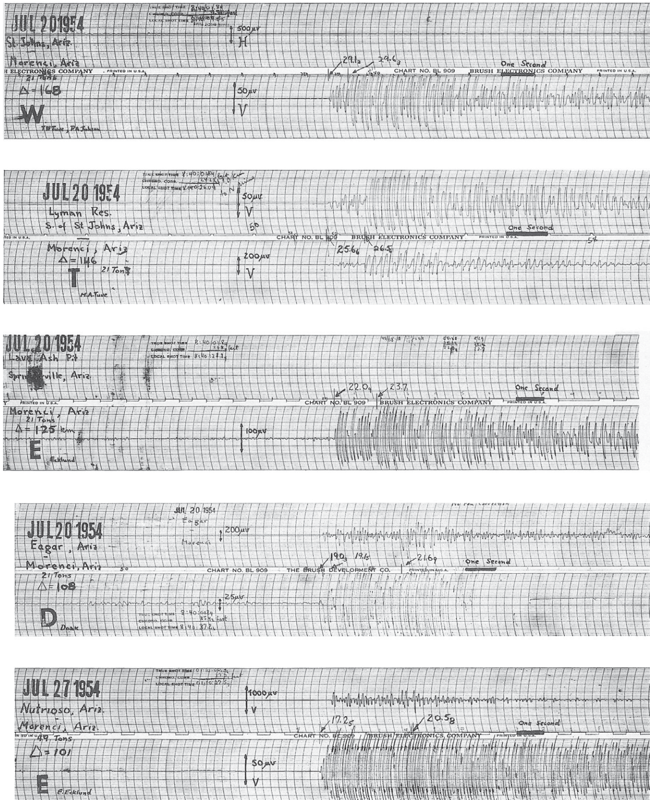
Figure 5.2-01. Field seismograms with critical reflections PP (3.2 to 0.5 seconds after first arrival from bottom to top seismogram) obtained in the Colorado Plateau in 1954 (from Tatel and Tuve, 1955, plate 5). [Geological Society of America Special Paper 62, p. 35–50. Reproduced by permission of the Geological Society of America.]
