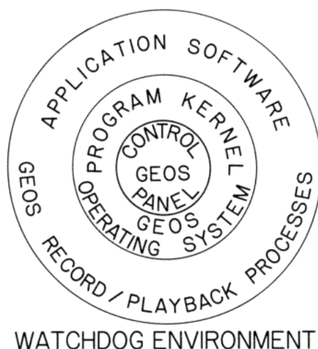
FIG. 6. Nested-ring structure of GEOS software architecture, showing inner ring containing system start-up and online debugging (see Figure 7), second ring containing GEOS operating system (see Figure 8), and third ring containing application software (see Figure 9), each of which is operated in a "watchdog" environment.
