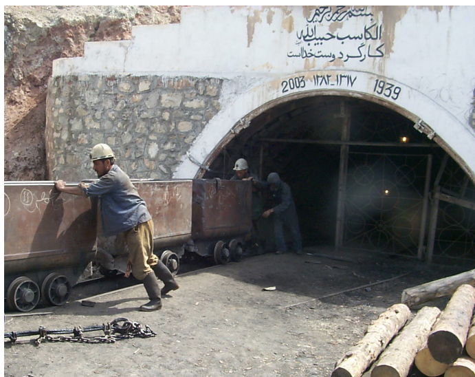
Figure 2. Karkar Mine, Baghlan Province. This North Coal Department mine, owned and operated by the Afghan government, is currently operating far below prewar (1978) capacity. The mine ventilation system is no longer fully functional, electric railcars have been replaced by winches, and expensive imported timbers are being used for roof support in place of local materials, which are no longer available.
