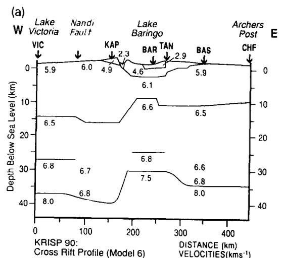
Fig. 3. Crustal and uppermost mantle velocity and interface model for (a) the cross profile, line D, and (b) the axial profile as obtained from raytracing (taken from KRISP Working Group, 1991a).
