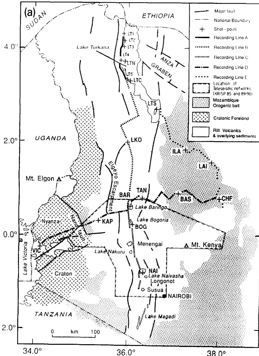
Fig. 1. (a) Tectonic map of Kenya including the location of the refraction profiles as well as the teleseismic arrays of KRISP85 and KRISP89/90. (b) Map showing the station locations of the 1985 and 1990 KRISP teleseismic programs including the proposed accommodation zones (Bosworth et al., 1986).
