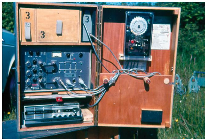
Figure 6.2.1-06. Recording unit MARS 66 equipped with a mechanical clock (upper right) (photograph by C. Prodehl). Upper left: T75A time-signal receiver; middle left: modulator; lower left: tape recorder. FS-60 seismometers in the background to the right.
