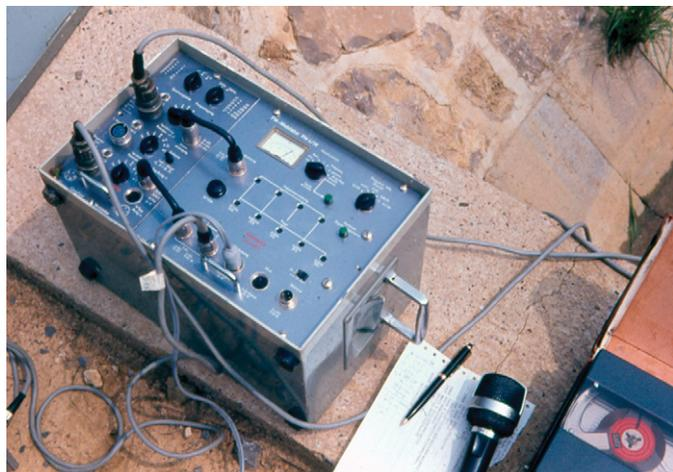
Figure 6.2.1-05. Recording unit MARS 66 (photograph by C. Prodehl). Left: modulator, lower right: tape recorder.
