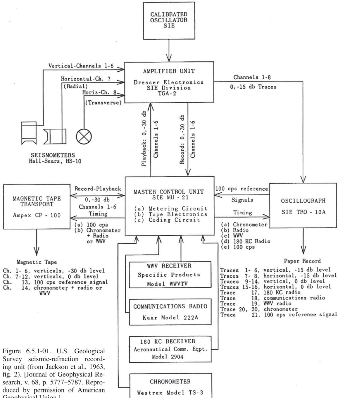
Figure 6.5.1-01. U.S. Geological Survey seismic-refraction recording unit (from Jackson et al., 1963, fig. 2). [Journal of Geophysical Research, v. 68, p. 5777-5787. Reproduced by permission of American Geophysical Union.]
