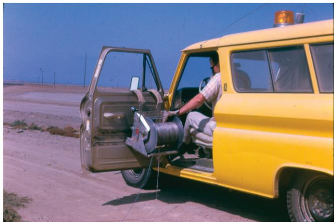
Figure 6.5.1-03. U.S. Geological Survey seismic-refraction recording truck, with Sam Stewart laying out an array of 6 seismometers (photograph by C. Prodehl).
