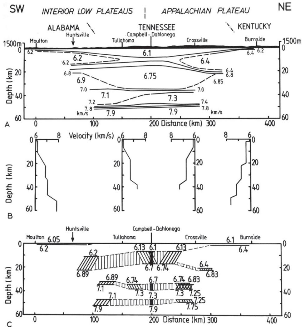
Figure 6.5.2-05. Crustal cross section between Moulton, Alabama and Burnside, Kentucky (from Prodehl et al., 1984, fig. 7). (A) Lines of equal velocity. (B) Individual velocity-depth profiles. (C) Position of velocity transition zones. [Tectonophysics, v. 109, p. 61–76. Copyright Elsevier.]
