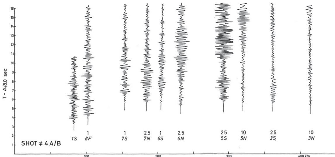
Figure 6.2.3-05. Seismogram section for line 7 (Fig. 6.2.3-02), southern shotpoint, along southeastern Norway, (from Kanestrom and Haugland, 1971, fig. 3). [In Vogel, A., ed., 1971, *Deep seismic sounding in Northern Europe*: Swedish Natural Science Research Council (NFR), Stockholm, 98 p. Permission granted by Swedish Research Council, Stockholm.]
