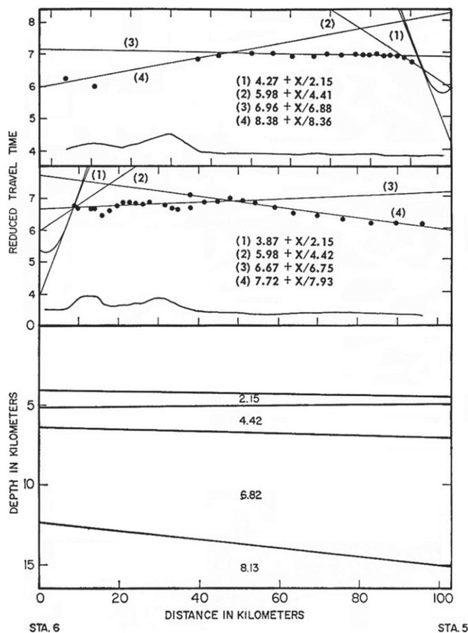
Figure 6.8.3-11. Traveltime plots and layer solutions for two of the Nova expedition reversing seismic refraction stations (from Shor et al., 1971, fig. 4). [Journal of Geophysical Research, v. 76, no. 11, p. 2562–2586. Reproduced by permission of American Geophysical Union.]
