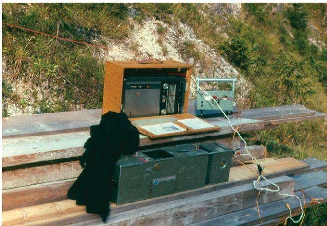
Figure 6.2.1-01. Mobile field station of the Institute of Applied Geophysics, University of Munich (photograph by C. Prodehl). The grey box below is the central recording unit with galvanometer and a photographic film device driven by a windshield wiper motor, top left: a radio receiver for time signal reception, top right: FS-60 seismometer.
