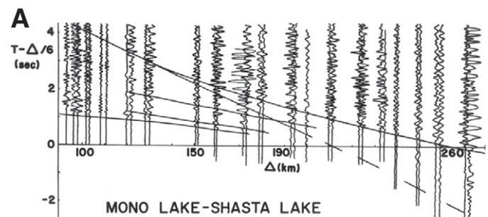
Figure 6.5.1-07. (A) Record section for the line Mono Lake to Shasta Lake, Sierra Nevada (from Prodehl, 1979, fig. 47). [U.S. Geological Survey Professional Paper 1034, 74 p. Copyright U.S. Geological Survey.] (Continued on following page.)
