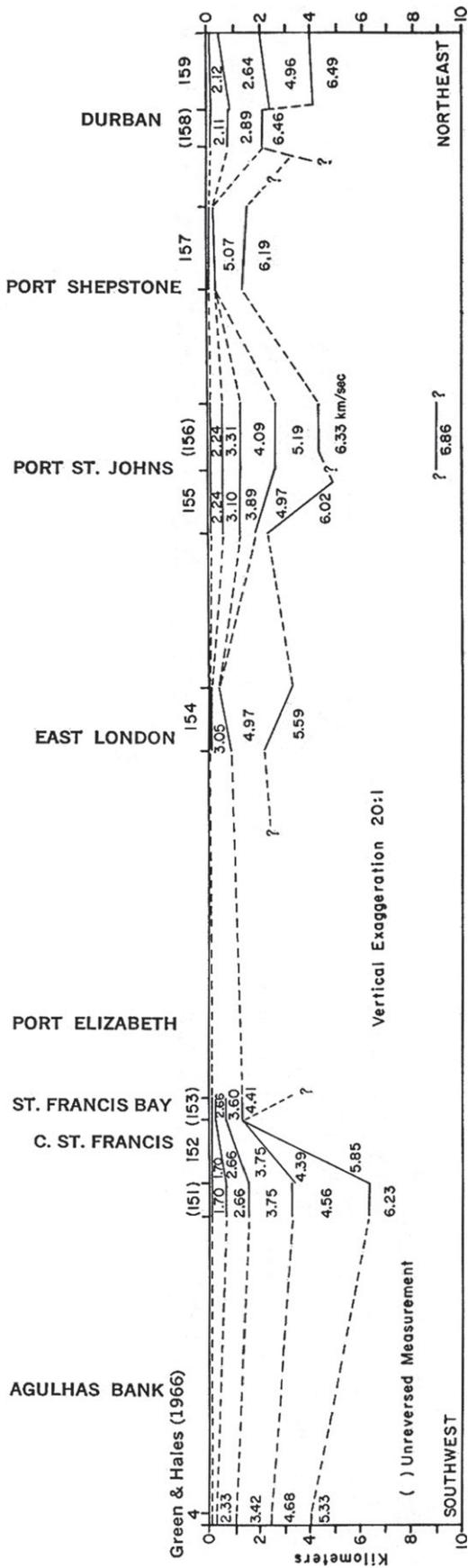
Figure 6.8.4-06. Seismic refraction section along the continental shelf between Agulhas Bank and Durban (from Ludwig et al., 1968, fig. 2). [Journal of Geophysical Research, v. 73, p. 3707–3719. Reproduced by permission of American Geophysical Union.]
