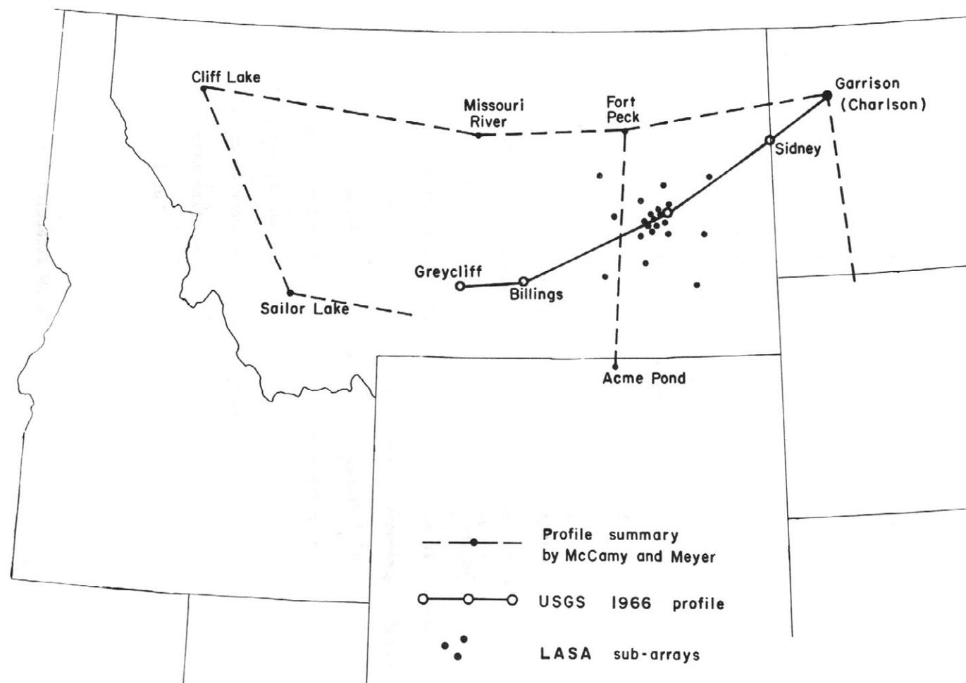
Figure 6.5.1-14. Seismic refraction, crustal calibration line, recorded across the LASA array in Montana in 1966 (from Warren et al, 1972, fig. 1). [U.S. Geological Survey Open-File Report, p. 1–58 and A1–A105.]
