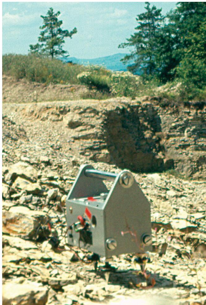
Figure 6.2.1-03. Electromagnetic seismograph constructed by H. Berckhmer, University of Frankfurt, Germany (photograph by C. Prodehl).
