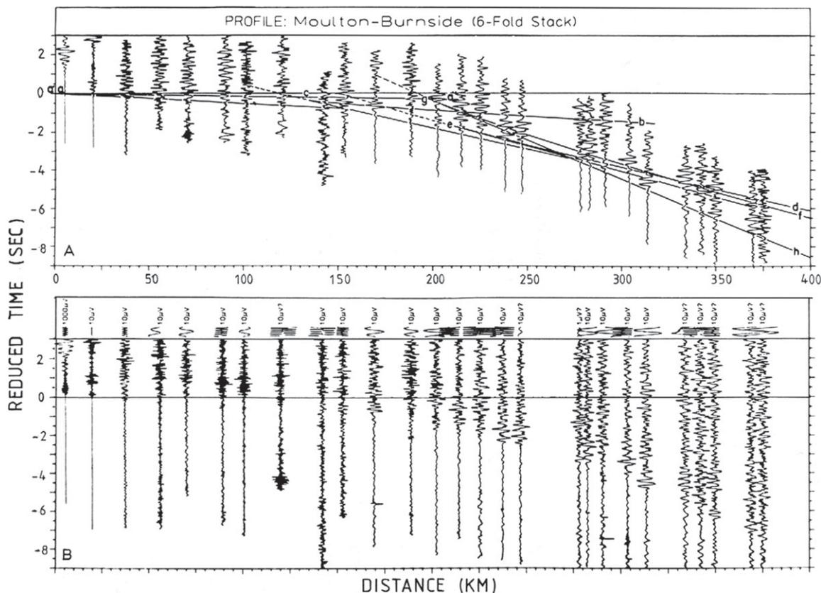
Figure 6.5.2-06. Record section of the profile Moulton–Burnside (from Prodehl et al., 1984, fig. 4). (A) Six-fold optimally stacked traces. (B) “Best” traces for each array. [Tectonophysics, v. 109, p. 61–76. Copyright Elsevier.]
