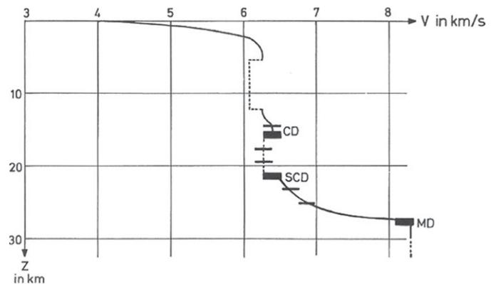
Figure 6.2.5-03. Near-vertical reflections (horizontal bars) in a velocity-depth curve from the Rhenish Massif (profile LO in Fig. 6.2.2-01) (from Meissner, 1973, fig. 10). Discontinuities: CD = Conrad, SCD = sub-Conrad, MD = Moho. [Geophysical Surveys, v. 1, p. 195-216. Reproduced by kind permission of the author.]
