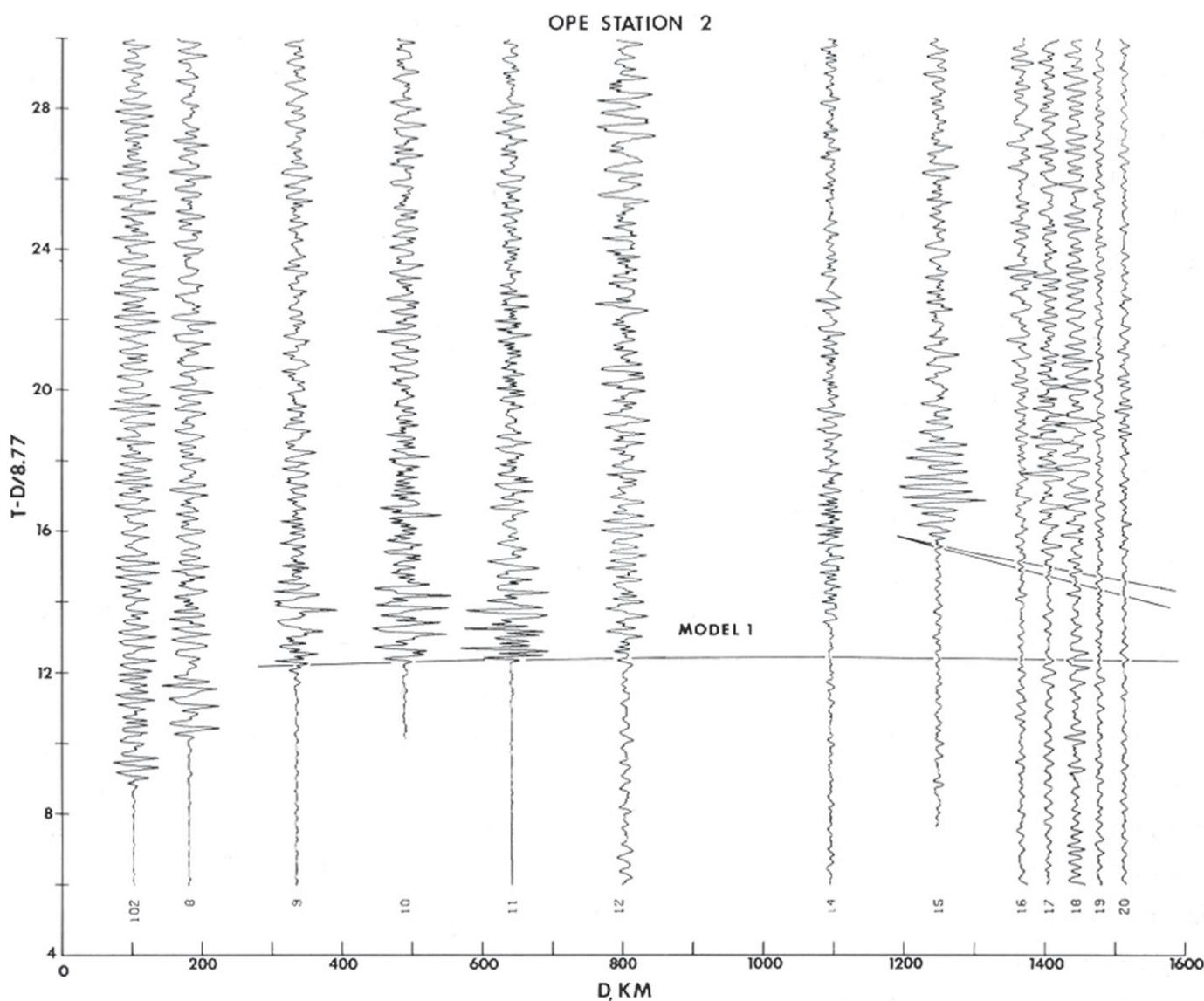
Figure 6.8.2-03. Record section of observations along the O.P.E. large-scale seismic refraction line of 1969 in the Gulf of Mexico (from Hales, 1973, fig. 4). [Tectonophysics, v. 20, p. 217–225. Copyright Elsevier.]
