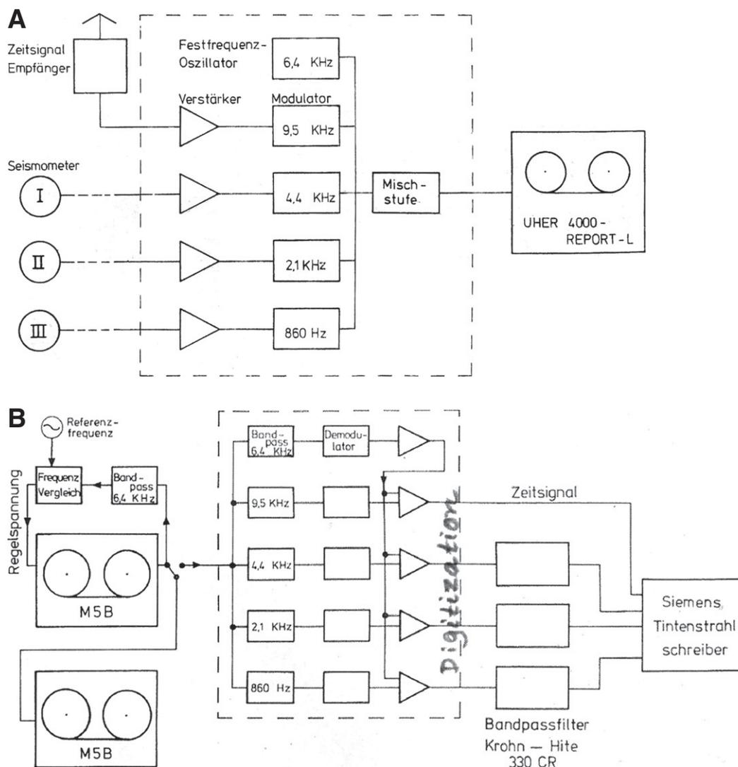
Figure 6.2.1-04. (A) block diagram of the recording unit MARS 66. (B) Block diagram of the playback unit (from Berckheimer, 1970, figs. 4 and 5). [Zeitschrift für Geophysik, v. 36, p. 501–518. Reproduced with kind permission of Springer Science+Business Media.]
