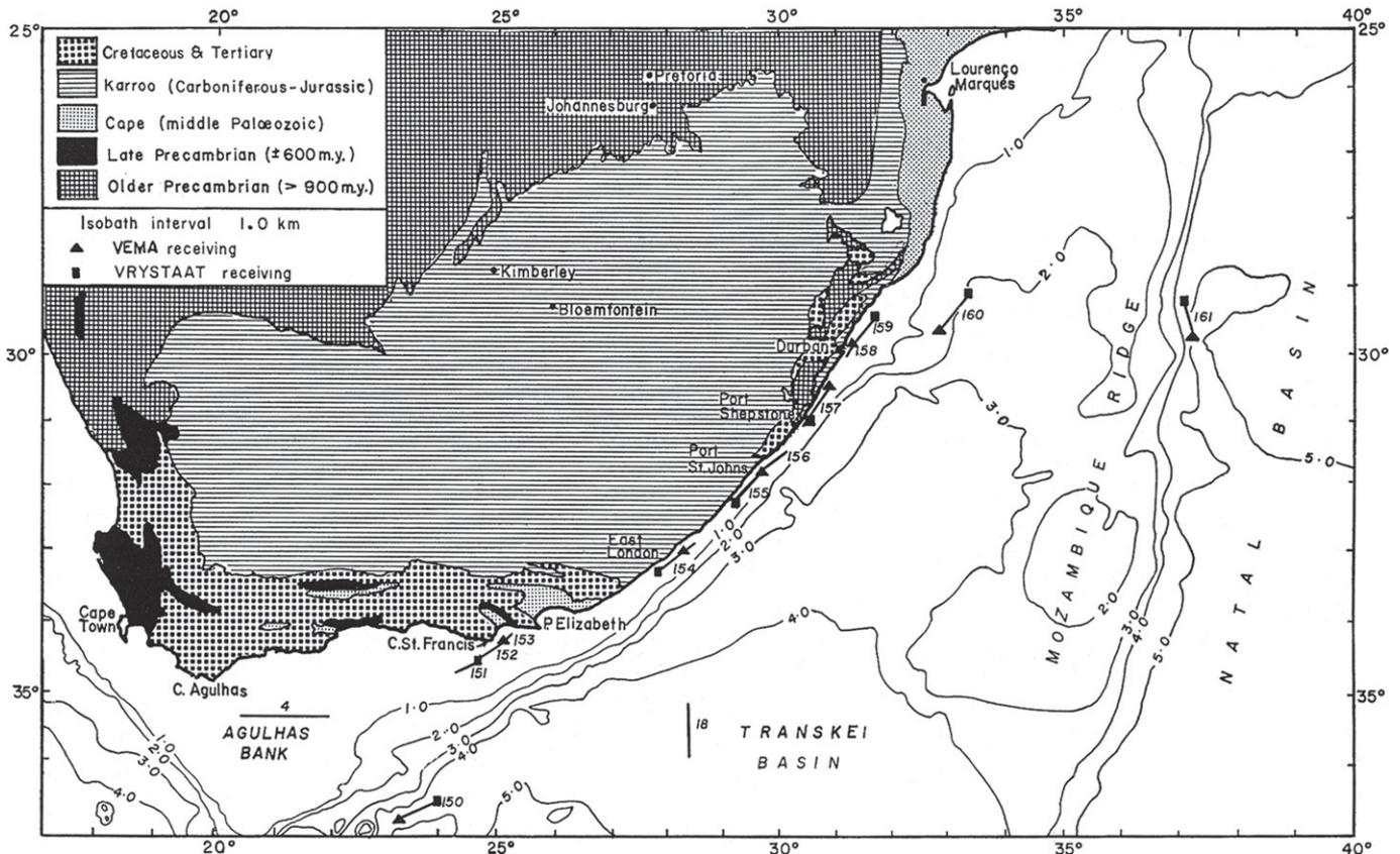
Figure 6.8.4-05. Simplified geological map of southeastern Africa showing the locations of offshore seismic refraction profiles (from Ludwig et al., 1968, fig. 1). [Journal of Geophysical Research, v. 73, p. 3707-3719. Reproduced by permission of American Geophysical Union.]
