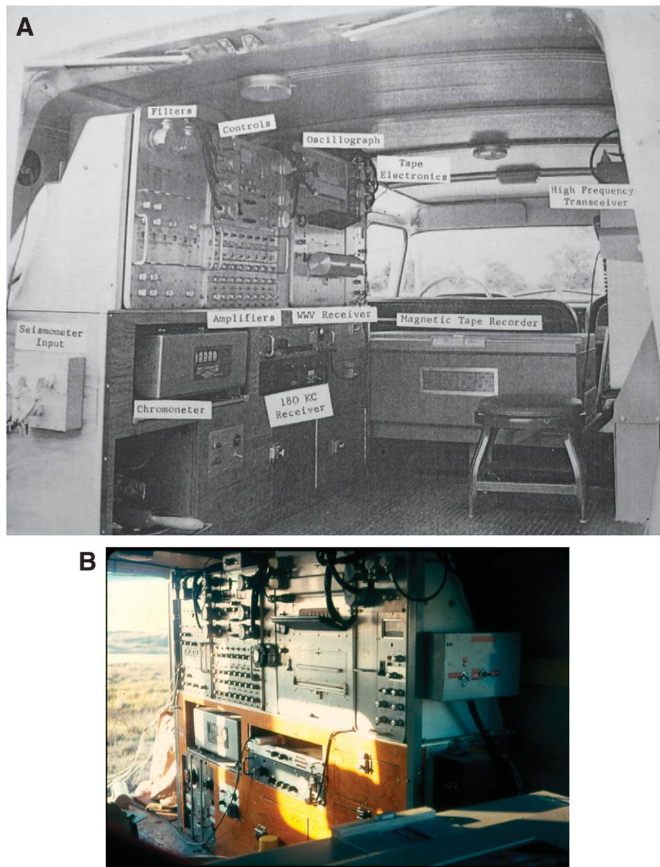
seismic and two timing channels, which allowed a 2.5-km-wide array of 6 vertical seismometers (with natural frequencies of 1–2 Hz) with average spacing of 500 m where terrain permitted, while two horizontal seismometers were usually placed in the center. Additional traces were available for recording the time signals of the broadcast station WWV, a calibrated chronometer, and when possible the shot instant. The details of this new seismic system were discussed by Warrick et al. (1961).
