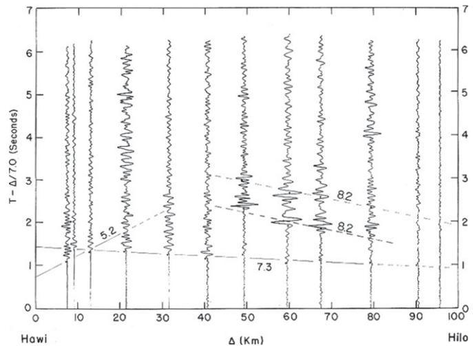
Figure 6.8.3-06. Record section of observations of a station located at the northern edge of the island of Hawaii (corresponding to position 5 of Fig. 6.8.3-04) and its recordings of shots along the northeastern coast of the main island of Hawaii (from Hill, 1969, fig. 5). [Bulletin of the Seismological Society of America, v. 59, p. 101–130. Reproduced by permission of the Seismological Society of America.]
