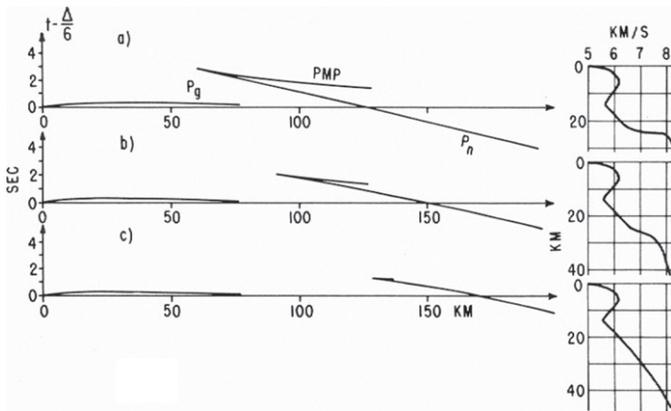
Figure 6.2.5-02. Traveltime diagrams and corresponding models for different structures of the crust-mantle boundary (after Giese, 1968, from Prodehl, 1977, fig. 1). [In Heacock, J.G., ed., The earth's crust: American Geophysical Union Geophysical Monograph 20, p. 349-369. Reproduced by permission of American Geophysical Union.]
