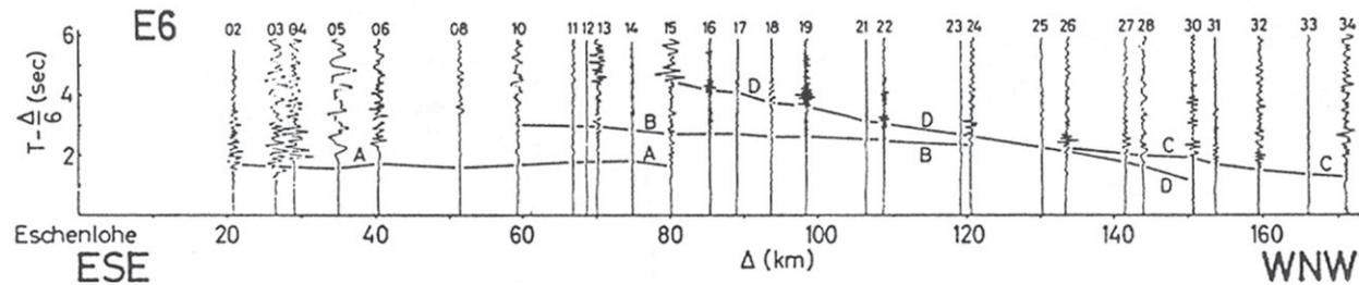
Figure 6.2.2-06. Record sections of data recorded from quarry blasts near Eschenlohe (01 in Fig. 6.2.2-01) across southern Germany (from Prodehl, 1965, figs. 4–9) [Bollettino di Geofisica Teorica e Applicata, v. 7, p. 35–88. Reproduced by permission of Bollettino di Geofisica, Trieste, Italy.]
